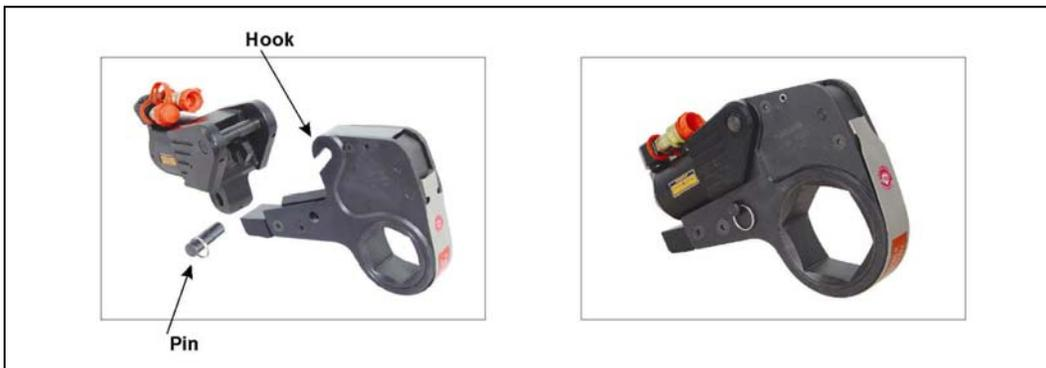
align. Insert the link pin to secure.
